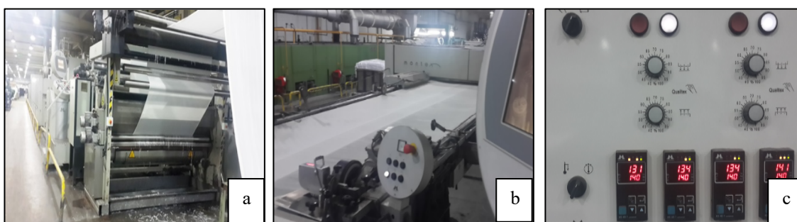
Figure 1 a- Fulard part, b- Fabric entrance to the cabinet, c- control unit Schematic representation of the stenter.
