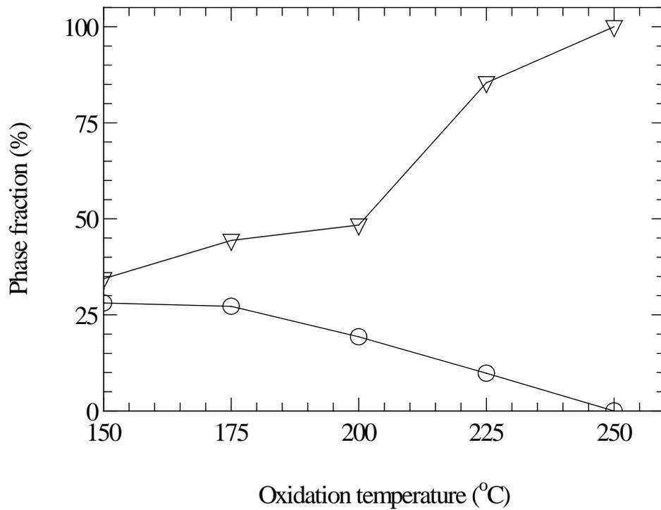
**Figure 9.** Variation of phase fractions of phosphoric acid pretreated and oxidized viscose rayon fibers as a function of oxidation temperature. (▽) amorphous phase; (○) crystalline (cellulose II) phase.
