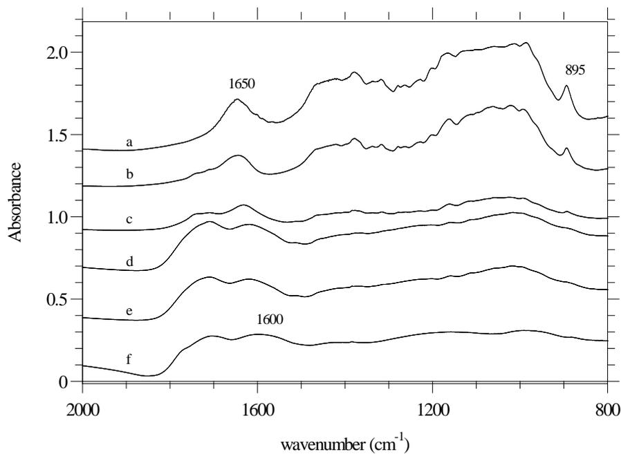
**Figure 12.** Infrared spectra of untreated (a) and phosphoric acid pretreated viscose rayon fibers oxidized in the air for 30 min as a function of oxidation temperatures in the 2000-800  $\text{cm}^{-1}$  region. (b) 150 °C; (c) 175 °C; (d) 200 °C; (e) 225 °C; (f) 250 °C.
