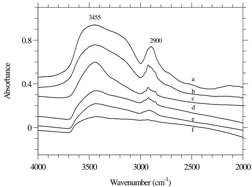
**Figure 11.** Infrared spectra of untreated (a) and phosphoric acid pretreated viscose rayon fibers oxidized in the air for 30 min as a function of oxidation temperatures. (b) 150 °C; (c) 175 °C; (d) 200 °C; (e) 225 °C; (f) 250 °C.
