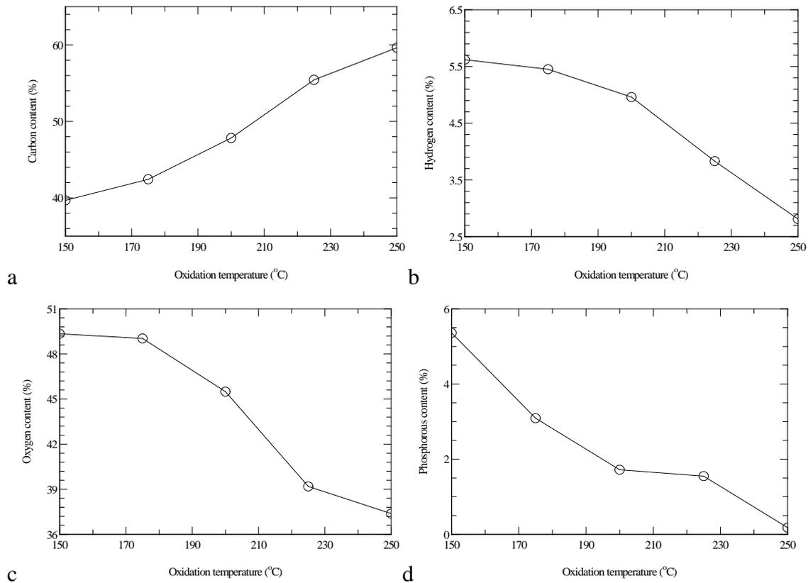
**Figure 2.** Elemental analysis of oxidized viscose rayon fibers pretreated with phosphoric acid as a function of oxidation temperature. (a) carbon (% wt.); (b) hydrogen (% wt.); (c) oxygen (% wt.); (d) phosphorous (% wt.).
