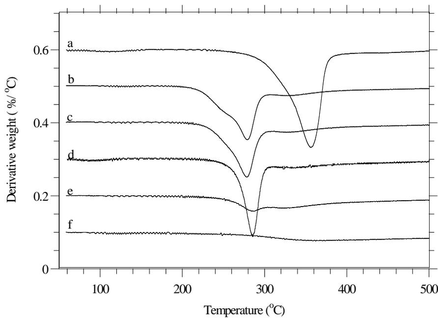
**Figure 6.** Derivative thermogravimetric curves of untreated (a) and phosphoric acid pretreated viscose rayon fibers oxidized at (b) 150 °C, 30 min; (c) 175 °C, 30 min; (d) 200 °C, 30 min; (e) 225 °C, 30 min; (f) 250 °C, 30 min.
