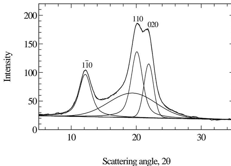
**Figure 8.** Curve fitting of equatorial X-ray diffraction trace of untreated viscose rayon fiber
