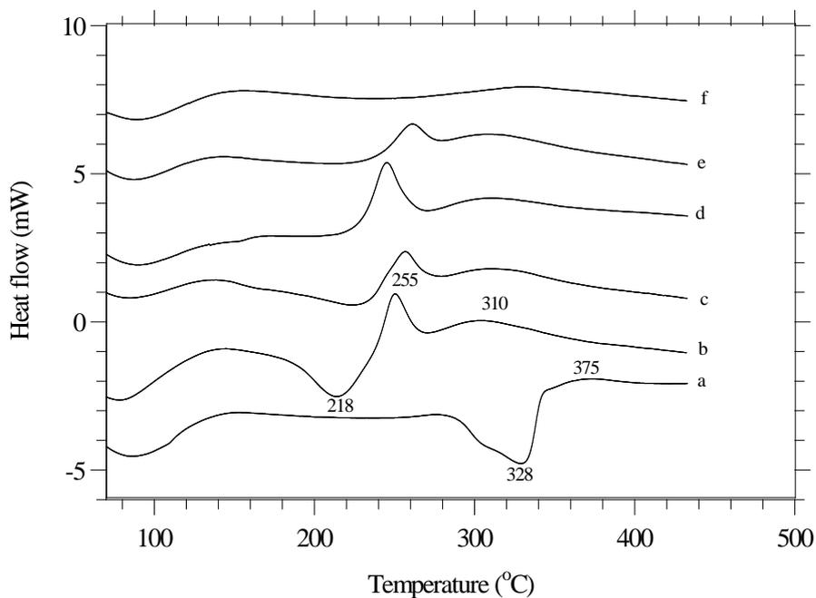
**Figure 4.** DSC thermograms of untreated (a) and phosphoric acid pretreated and oxidized viscose rayon fibers as a function of oxidation temperature. (b) 150 °C, 30 min; (c) 175 °C, 30 min; (d) 200 °C, 30 min; (e) 225 °C, 30 min; (f) 250 °C, 30 min.
