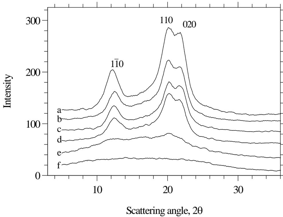
**Figure 7.** Equatorial X-ray diffraction traces of untreated (a) and phosphoric acid pretreated viscose rayon fibers oxidized at (b) 150 °C, 30 min; (c) 175 °C, 30 min; (d) 200 °C, 30 min; (e) 225 °C, 30 min; (f) 250 °C, 30 min.
