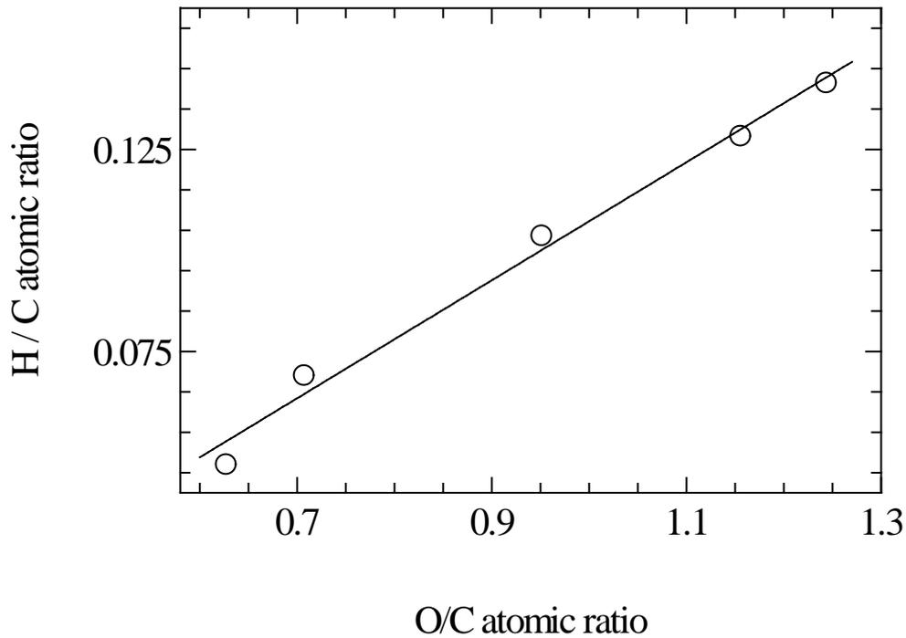
**Figure 3.** Comparison of H/C against O/C atomic ratios for the phosphoric acid pretreated and oxidized viscose rayon fibers as a function of oxidation temperature.
