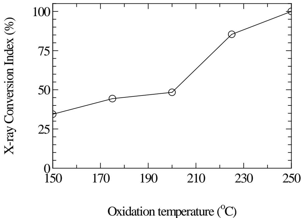
**Figure 10.** Variation of X-ray conversion indices of untreated and phosphoric acid pretreated and oxidized viscose rayon fibers as a function of oxidation temperature.
