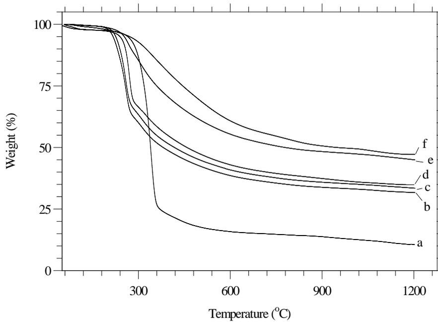
**Figure 5.** TGA thermograms of untreated (a) and phosphoric acid pretreated viscose rayon fibers oxidized at (b) 150 °C, 30 min; (c) 175 °C, 30 min; (d) 200 °C, 30 min; (e) 225 °C, 30 min; (f) 250 °C, 30 min.
